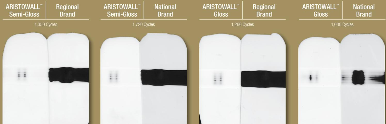
Test Method: Paints are applied to black charts. After drying for seven days, the charts are placed in an abrasion testing machine and stopped at the indicated cycle. Complete film deterioration occurs when a full line of black background is exposed.
